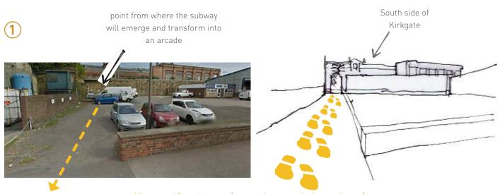
New **south entrance** (extension to existing subway). The level at the bottom of the subway aligns with the ground level on the south side of the station.
